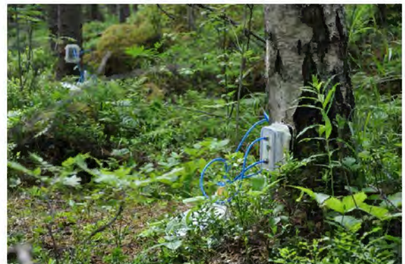
Chambers attached to trees to measure N 2 O emissions
